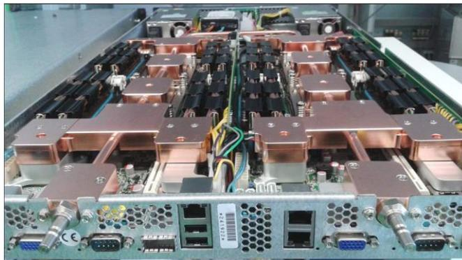
*Figure 3 Server with on-chip liquid cooling system*
