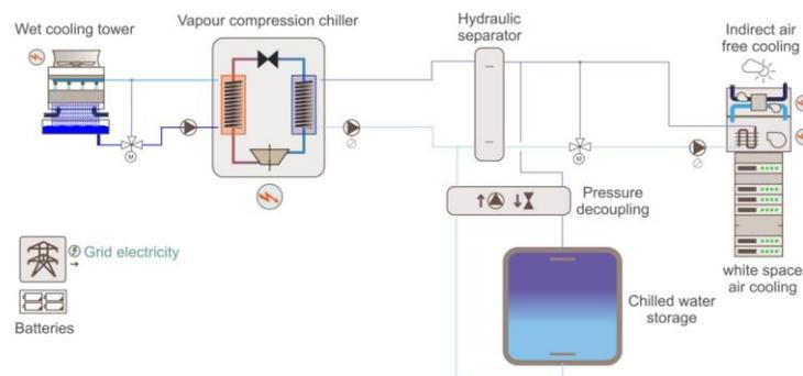
Figure 6 Thermal scheme of a data centre with thermal and electrical energy storages
