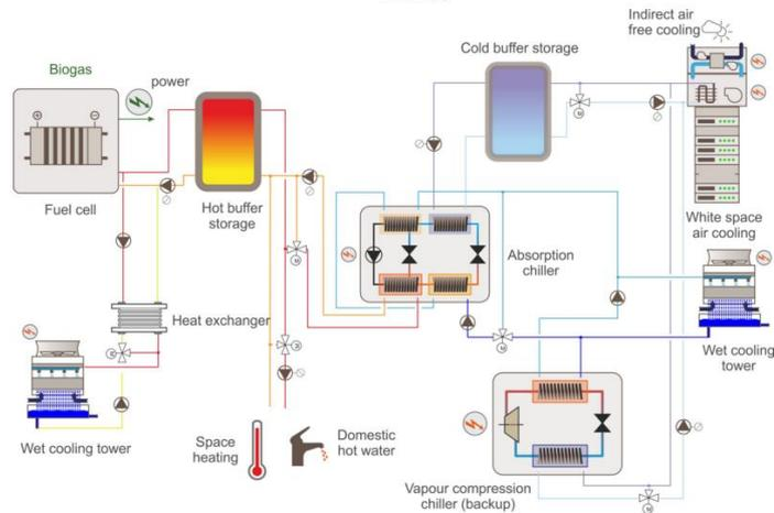
*Figure 7 Thermal scheme of a data centre with a biogas fuel cell and absorption chiller.*
