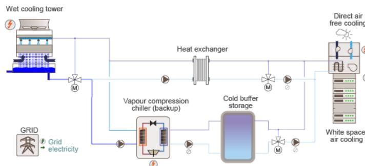
Figure 5 Thermal scheme of a data centre with wet cooling towers
