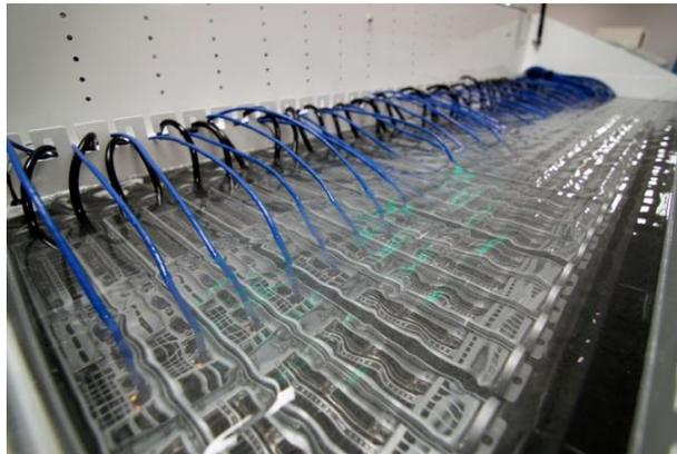
Figure 4 Immersed racks on a nonconductive fluid. Source: *technologyreview*<sup>1</sup>
