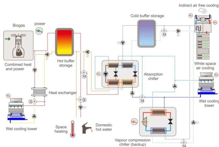
*Figure 8 Thermal scheme of a data centre with a reciprocating engine CHP and absorption chiller.*
