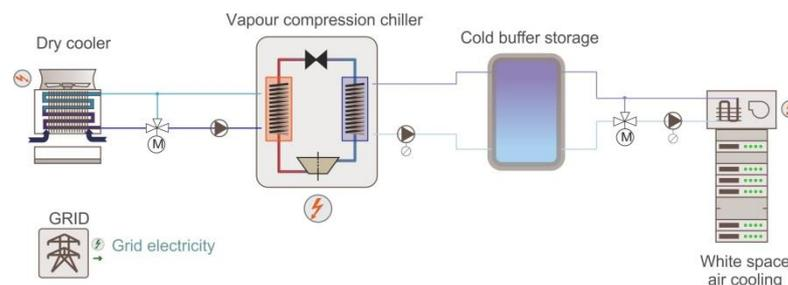
*Figure 1 Thermal scheme of a conventional data centre*
