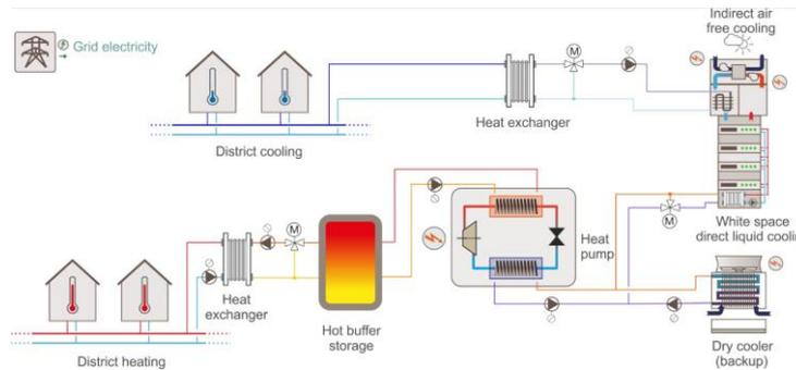
*Figure 2 Thermal scheme of a data centre connected to a district cooling and heating network and with direct liquid cooling system*
