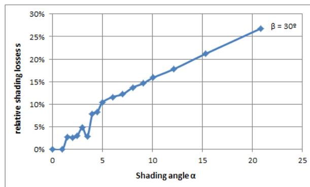
Figure 4 Relative shading losses for a 30° panel tilt at locations with latitudes higher than 55°.
