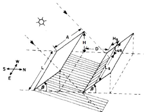
Figure 1 Geometric relation between panel tilt, row space and solar height.
