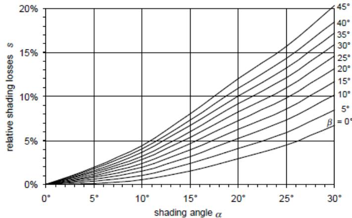
Figure 3 Relative shading losses for different panel tilts at locations with latitudes between 45-55° [8].
